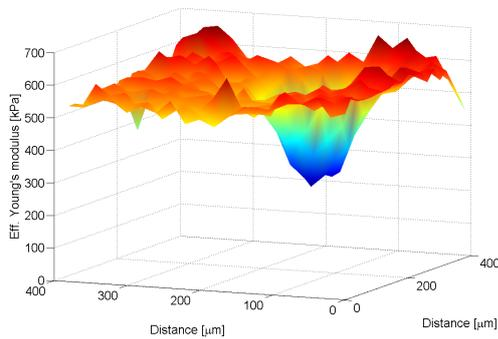
**Figure 1:** 3D elasticity map of a 25 x 25 point grid scan of 4% LMP agarose. The point-to-point pitch is 25  $\mu\text{m}$ .
