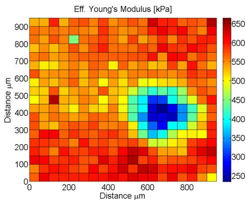
**Figure 2:** 2D elasticity map of a  $25 \times 25$  point grid scan of 4% LMP agarose. The point-to-point pitch is 25  $\mu\text{m}$ .
