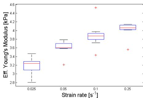
**Figure 6:** Boxplot of effective Young's Modulus estimates for different strain rates. Strain rates 0.025, 0.05, 0.1 and  $0.25 \text{ s}^{-1}$  correspond to 0.92, 1.82, 3.64 and  $9.13 \text{ μm/s}$  displacement velocities, respectively.
